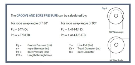
Safe design practice uses 3,000 psi in both the bore and groove as maximum pressure allowable. The groove pressure can withstand 4,000 psi for limited periods of time, but the bore pressure should remain limited at  $\leq$  3,000 psi.
